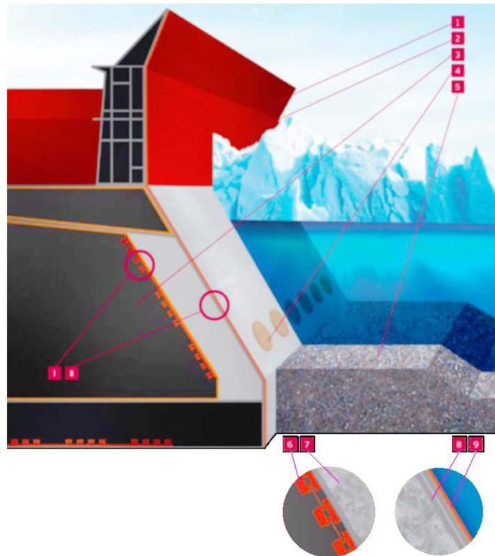
**Figure 3—Design of the caisson in the section: 1 - wave deflector, 2 - ice deflector, 3 - resistant paint coating of oil storage tanks, 4 - electrical corrosion protection, 5 - bulk soil layer, 6 - protection against corrosion, 7 - concrete 3 m thick, 8 - double-layer steel sheet, 9 - cladding with stainless steel. Рис. 4. 3D схема кессона. Source: PJSC Gazprom Neft.**
