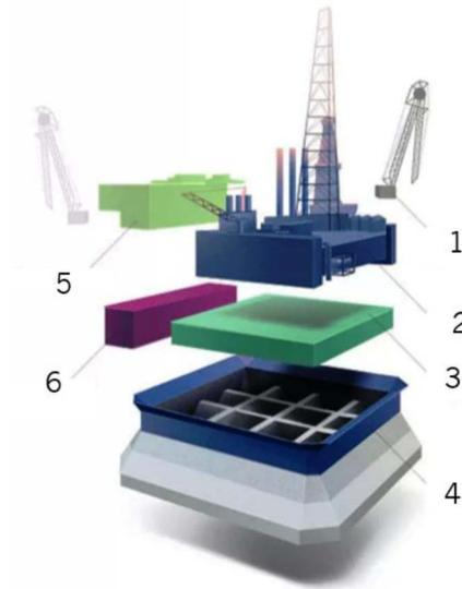
**Figure 2—Schematic representation of a platform structure with a caisson, where 1 - shipment module; 2 - upper structure; 3 - intermediate deck; 4 - caisson; 5 - additional module; 6 - auxiliary module. Source: PJSC Gazprom Neft.**
